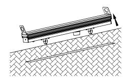
Follow installation instructions carefully. Ensure all below ground termination is totally sealed. Do not shorten the cable lengths
