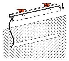
2) Ensure that the fixings (3) are Horizontal and flat. The base must be locked in place by a binder, be that silicone or concrete. Wait for the binder to set.
