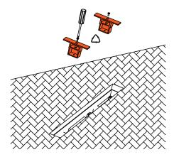
4) Take the head (1) ensuring the probe matches inside the channel (4) and place the head in place ensuring this is correctly located.
