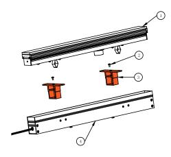
Cut a Channel to the size of the aluminium base (4). Connect the
