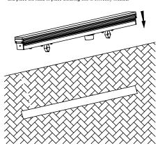
5) To remove the head use the additional removal brackets. Locate one at either end and pull at same time to remove.
