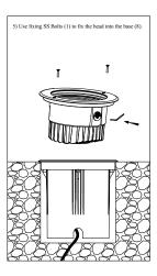
Follow installation instructions carefully. Ensure all below ground termination is totally sealed. Do not shorten the cable lengths provided on the fixture. Ensure all power is Off during installation until circuit is complete.
