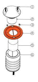
Core Drill a hole in the ground. Insert base (6) into said hole with concrete/Silicone if required. Connect the power lead to Gel sealed connector, ensuring no cable lengths are cut on the fitting. Ensure part (6) is sat horizontally. With fixing plate (4) above the surface.
