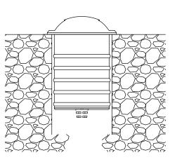
Follow installation instructions carefully. Ensure all below ground termination is totally sealed. Do not shorten the cable lengths provided on the fixture. Ensure all power is Off during installation until circuit is complete.
