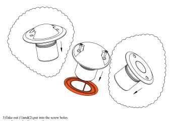
4)PLace the head into the base and fix with the two SS bolts provided (1).
