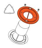
2) Once Concrete/Silicone is set correctly and ensuring the base is horizontal remove the fixing plate (4).Ensure the inside of the base is clean.
